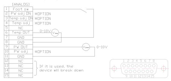
•It is necessary to use a Shielded Cable and a ferrite core for this connection.
