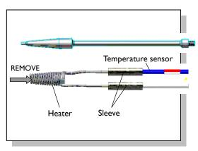
**6.** Check the contact between the tip and the heater. If the heater position is too much forward or if the heater is pressing too much on the tip, adjust so they are not in contact with each other. The guideline for adjustment is to have the end of the heater coiling and the begining of the straight section of the tip matching.
